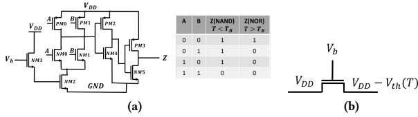
Figure 3: (a) Polymorphic NOR/NAND gate functioning as NOR for T greater than T_B , and as NAND for T less than T_B . V_b is applied voltage controlling temperature threshold T_B . (b)NFET threshold effect due to temperature. V_b is the variable gate voltage, which can be adjusted depending on the desired temperature threshold in our polymorphic gates.
