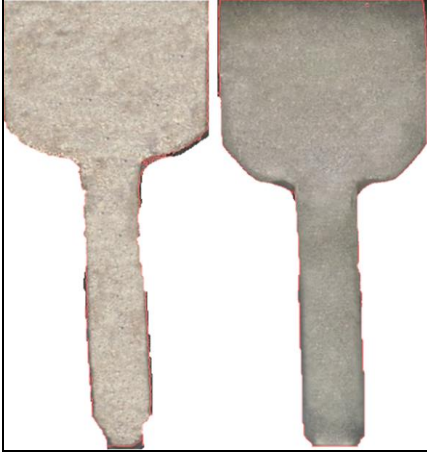
Figure 5: Result of segmentation on pins without any corrosion.
