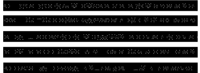
Figure 17: Image showing strips of contact extracted from the binarized image. The V_{cc} supply lines in the image are removed after detection
